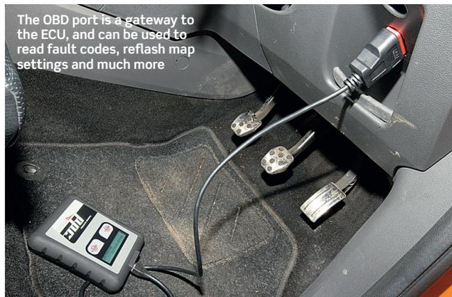
The OBD port is a gateway to the ECU, and can be used to read fault codes, reflash map settings and much more
