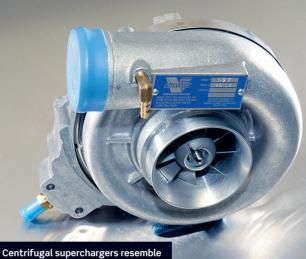
Centrifugal superchargers resemble the snail-like shape of a turbo
