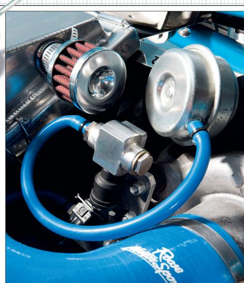
Air injectors can be used to precisely control the actuator
