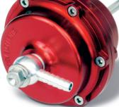
a wastegate actuator. This is simply bolted to the turbo itself. It consists of a metal canister with a spring and diaphragm inside it connected to a rod which is in turn connected directly to the wastegate arm. Inside the canister, the incoming boost signal pushes on the diaphragm and compresses the spring. The more pressure (boost) that enters the actuator, the further out the rod is pushed and the further the wastegate opens. Simple.
