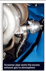
like CV boots and rubber brake lines, simply because they are not directed to a suitable area. So think carefully when having one fitted and exercise some common sense. A screamer pipe is a flamethrower... please treat it like one.
