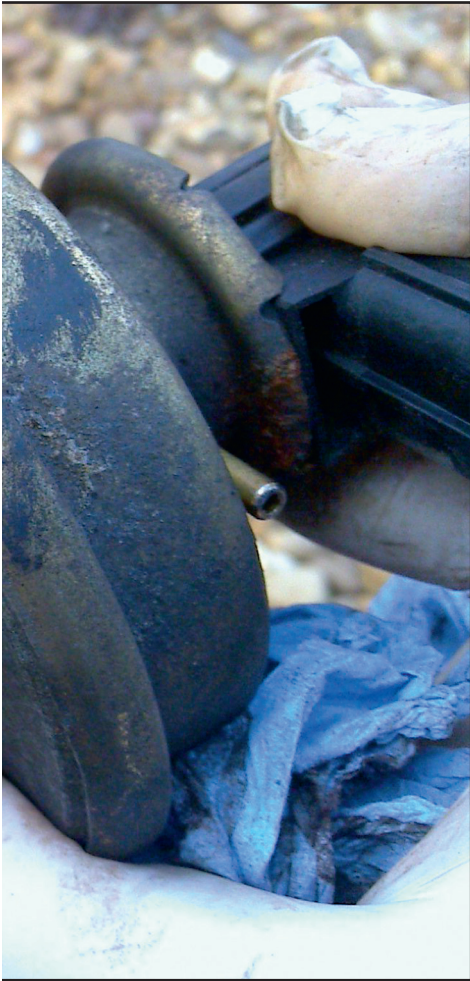
The plunger valve can be seen inside the EGR
