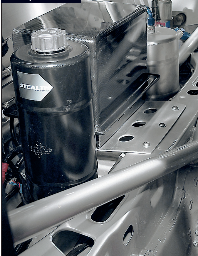
Water injection tanks are often mounted alongside the fuel system
