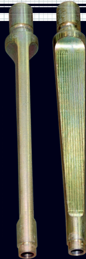
Bladed roll bars are infinitely adjustable between horizontal, the full soft setting, and 90deg vertical, the full hard setting
