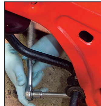
Anti-roll bars are usually fixed directly to the chassis by at least two fixing points
