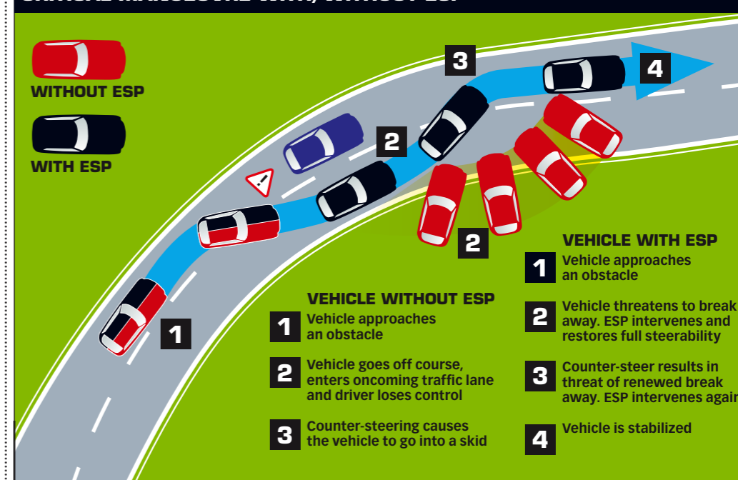
ESP uses input from wheels and steering wheel angle sensors
