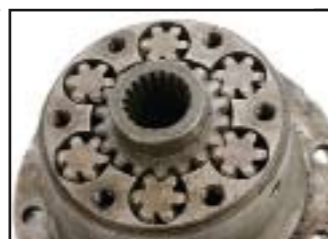
Geared diffs like the ATB use worm gears to transfer torque
