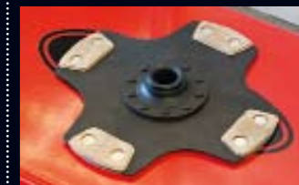
Paddle or cermetallic clutches can handle increased torque but aren't suited to constant road use
