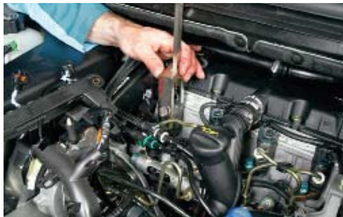
High-pressure pump supplies fuel to the 'common rail' at as much as 2000bar
