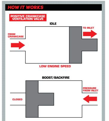
All crankcase ventilation systems work in a similar way. Up until around 1960 they used to just dump the vapours and oil out to the atmosphere via the filler cap, but due to strong pressure from environmental groups the systems were redesigned to find a way to keep all the vapours and waste oil inside the engine compartment, thus the PCV (Positive Crankcase Vantilation) system was born
