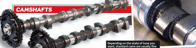
Contrary to popular belief the camshafts on a normally aspirated engine are normally quite good for a turbocharged application under most conditions.
