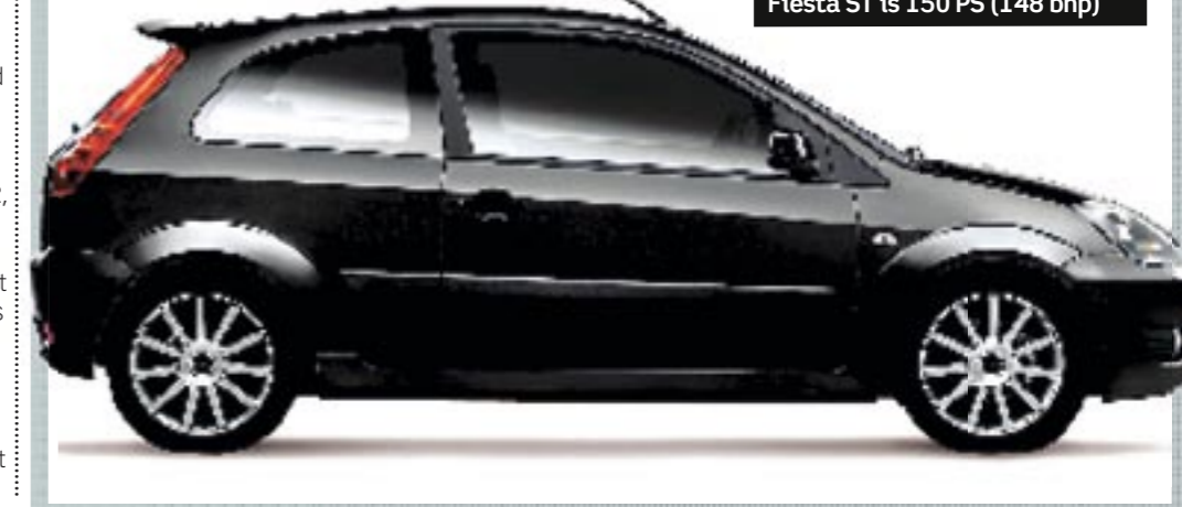
Most manufacturers now quote PS instead of bhp. Hence the Fiesta ST is 150 PS (148 bhp)
