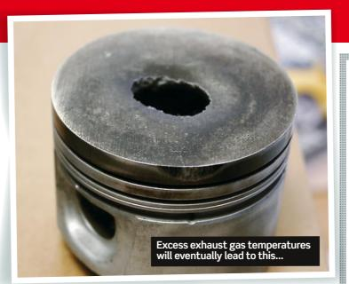
Engines with air flow meters (MAF systems) can compensate to a certain degree depending on how well programmed they are for such changes in the first place. Some are great, some are awful. Engines equipped only with map sensors (speed density) are in trouble and due to their very nature will definitely run leaner, providing the parts fitted do actually improve airflow. (For the reason why, please see Fast Ford issue 248.)
