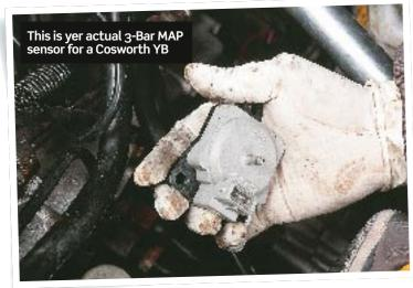
zero-5 volts, so your ECU on a 2 bar ECU program is set to understand that when the MAP sensor sees 15 psi at the intake plenum it will send out 5 volts and in turn the ECU will then inject enough fuel for 15 psi.
