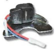
Crank position sensor (under bottom pulley)
