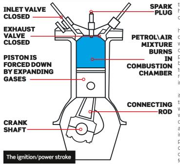
compressed to this immense level, our mixture of fuel and air becomes extremely volatile and a single spark from the spark plug will initiate the combustion of it and release the energy from the mixture, forcing our piston smoothly back down the bore and producing our next stroke — the power stroke.
