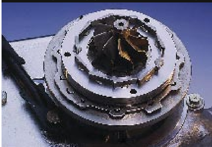
The future: this is the adjustable turbine housing from a variable-geometry turbo as found on Ford's 2-litre TDCi engine. These turbos can't cope with huge power levels, but it won't be long
