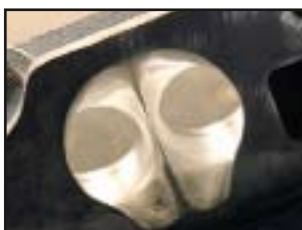
Porting the cylinder head improves airflow, making it suited to high revving applications
