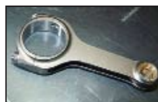
Forged con rods are a must for high revving engines
