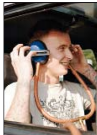
Det cans aren't fancy, but allow you to hear detonation or knock
