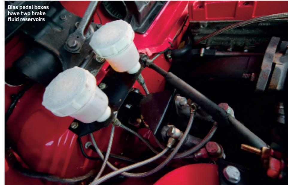
Bias pedal boxes have two brake fluid reservoirs
