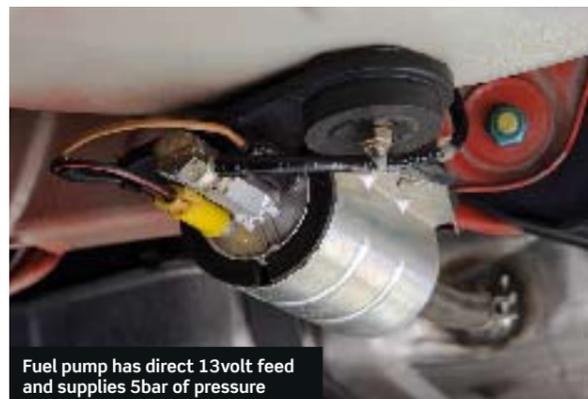
Fuel pump has direct 13volt feed and supplies 5bar of pressure
