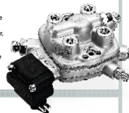
SENSOR PLATE MOVES AS AIR DEMAND IS INCREASED, ALTERING THE AMOUNT OF FUEL BEING DELIVERED
