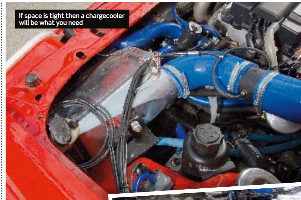
Chargecoolers have their own radiator for cooling the water
