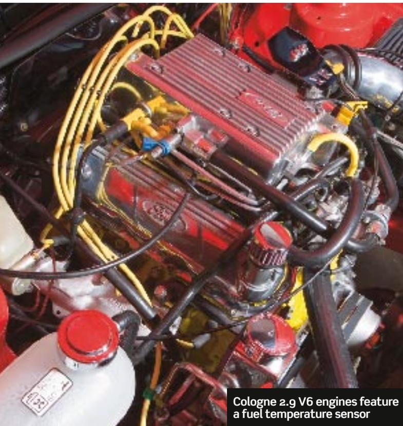
Cologne 2.9 V6 engines feature a fuel temperature sensor
