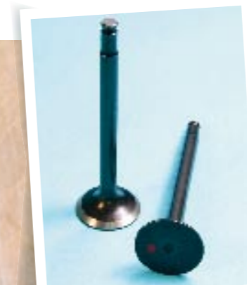
The valve size will greatly affect the choice of cam for your engine
