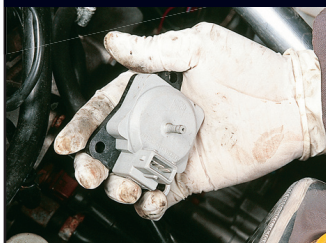
MAP sensors feed the ECU info about boost pressures
