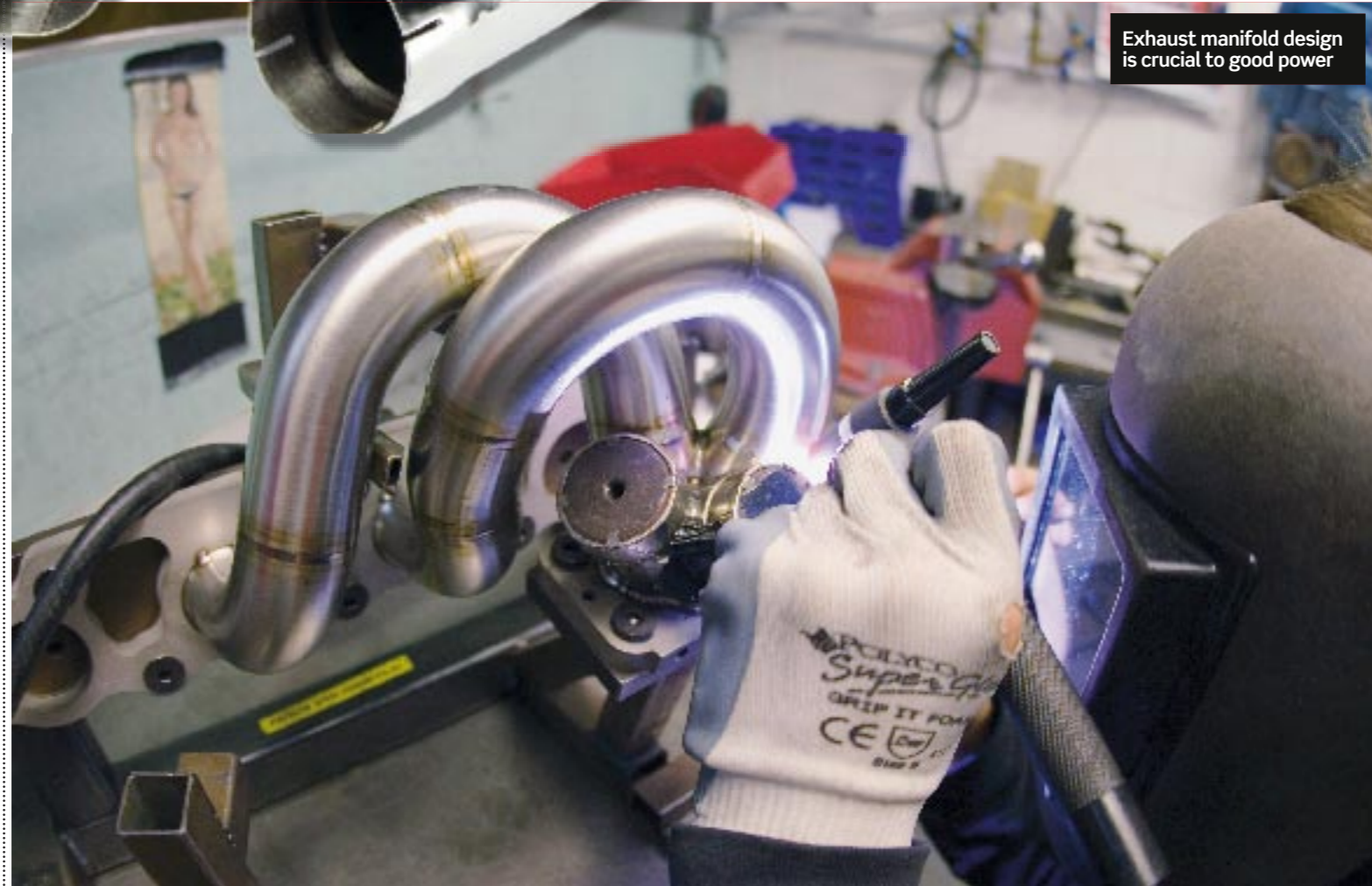
Equal-length primaries don't suit all engines
