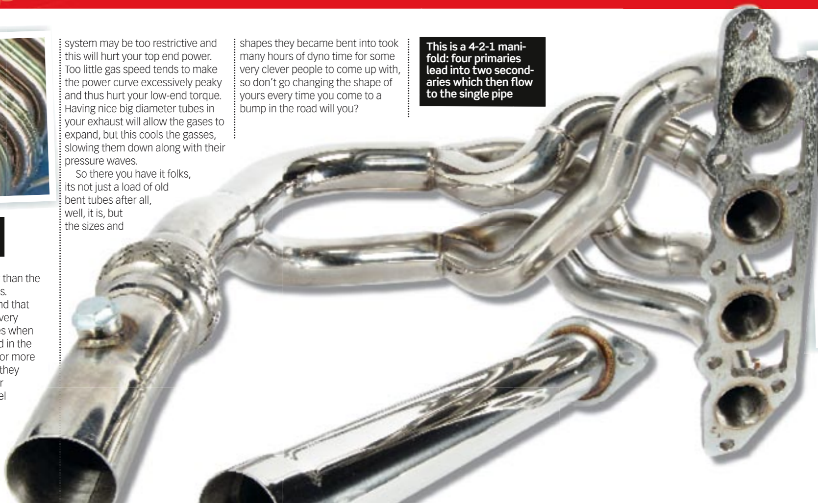
Exhaust manifold design is crucial to good power
