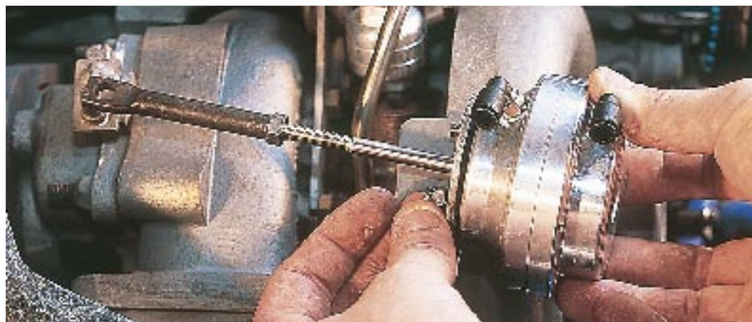
This is the wastegate actuator. The sealed canister contains a diaphragm and spring that act on the wastegate control arm on the turbo using the rod to hold the wastegate shut until required to open
