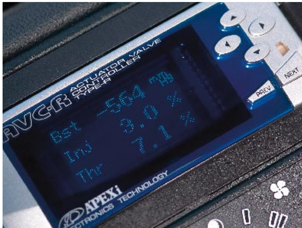
Dig the new breed: electronic boost controllers from Japan are finding their way into more and more big-power Fords. Tricky and expensive to fit, maybe, but they're the future for accurate boost control
