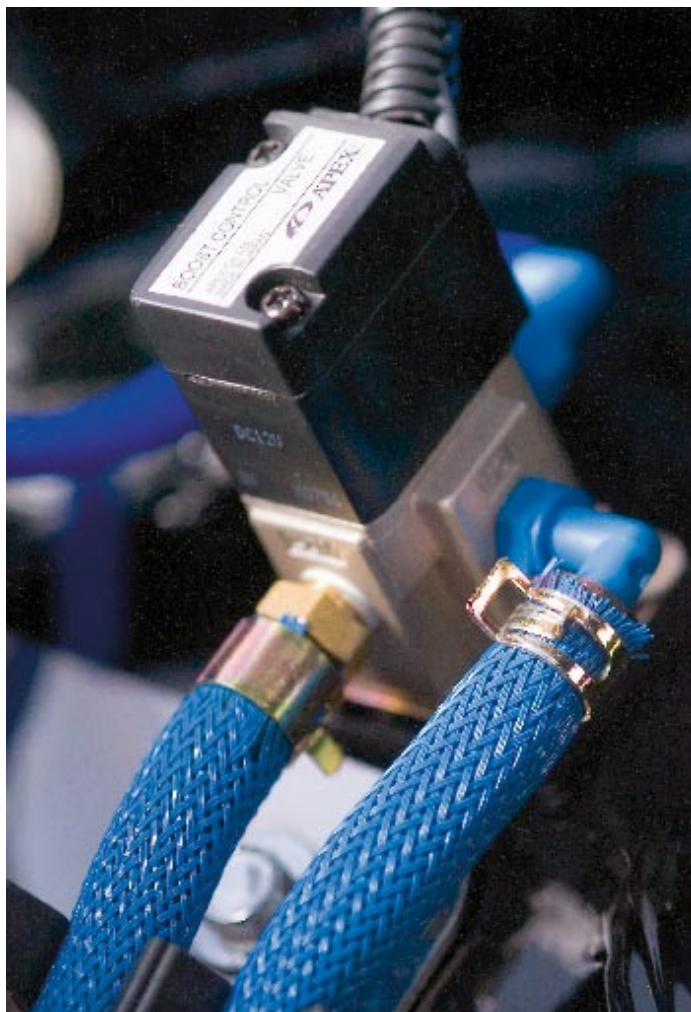
Electronic boost controllers (below) use one or two solenoids rather than injectors to control bleed off of boost pressure
