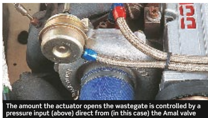
This is the wastegate actuator. The sealed canister contains a diaphragm and spring that act on the wastegate control arm on the turbo using the rod to hold the wastegate shut until required to open
