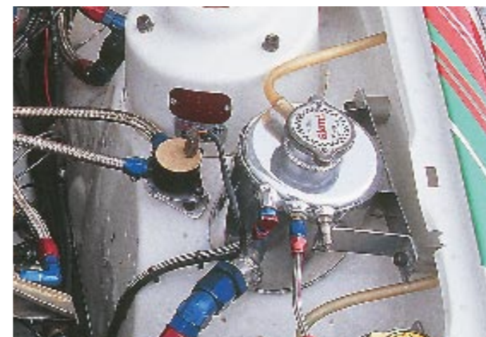
The Amal valve was fitted as standard to RS Turbos and Sierra Cosworths, and is a simple electronic bleed valve that works well
